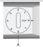
Turn off: rotate the knob back to position STOP (0). Setting the temperature
