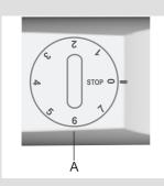
Turn off: rotate the knob back to position STOP (0).
